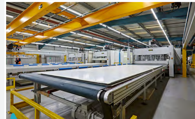
'SMART' GRP sidewall during the production process.
