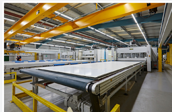
'SMART' GRP sidewall during the production process.
