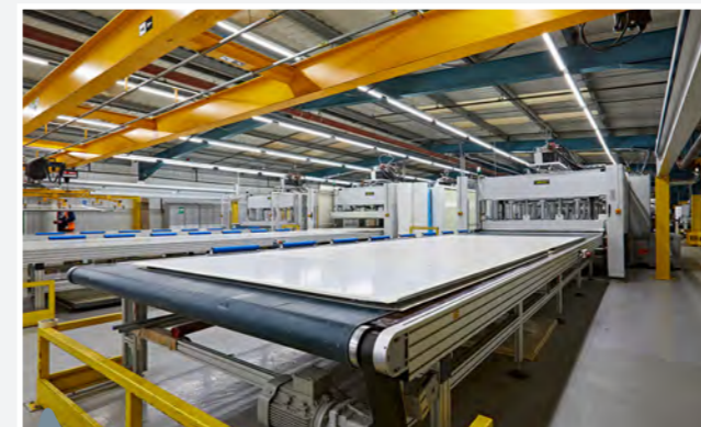
'SMART' GRP sidewall during the production process.
